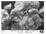
SEM image of lithium manganese oxide ( $LiMn_2O_4$ ) obtained using a modified solgel method.
