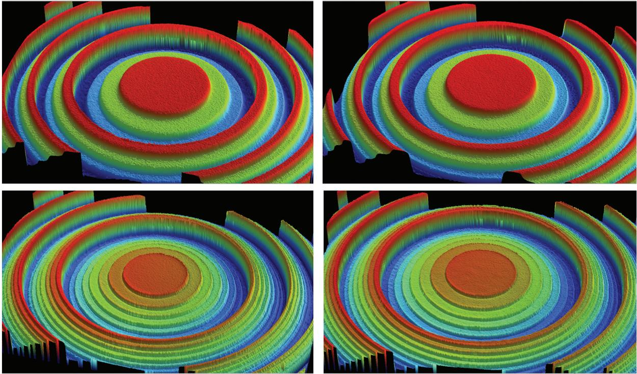
**Fig. 1.** Images of the central part of the four- and eight -phase-level diffractive lenses (top and bottom, respectively) (Veeco Contour GTK 1 optical profilometer): on the left – a quartz original, on the right – a replica on COC substrate.
