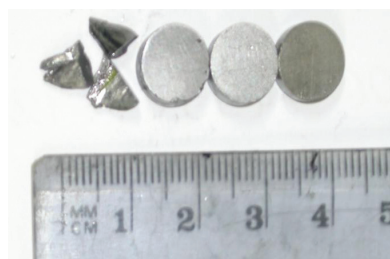
Fig. 17. BTI-2 crystal after cutting it into wafers of a thickness of approx. 4 \text{ mm} , destined for the structural and electrical measurements.
