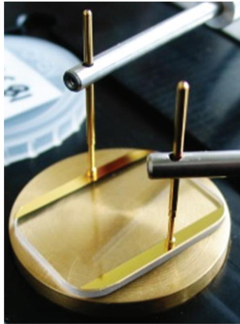
**Fig. 2.** Photograph of graphene-based heater deposited on glass plate.
